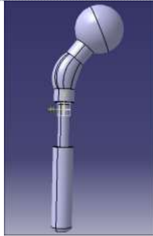
Fig. 1: Redesigned implant model from the parameters taken from the Paper probabilistic design of newly designed cemented hip prosthesis.
